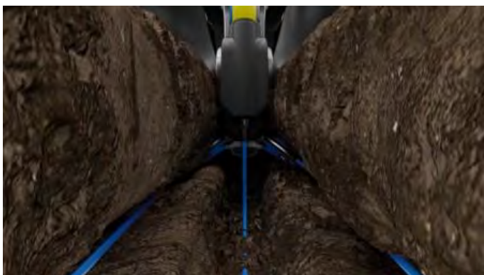
Figure 1. FurrowJet® Center and Wing Placement
