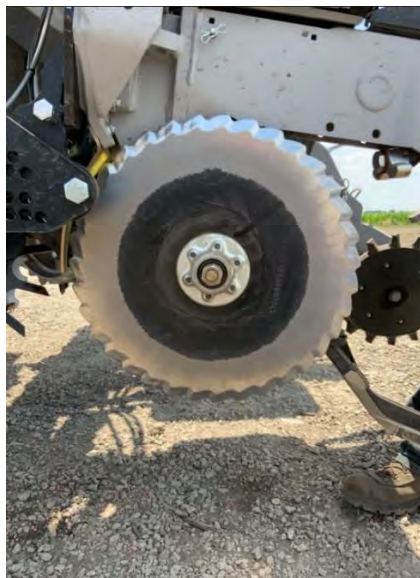
STP disc installed on International Harvest planter
