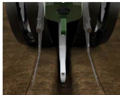
Figure 2. Conceal® Dual Placement 3" from Seed Furrow, 1.5" in Depth
