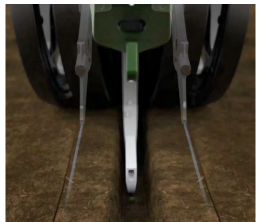
Figure 1. Conceal® Dual Placement 3" from furrow
