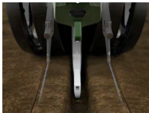
Figure 2: Dual Band Conceal® Out of Furrow Bands
