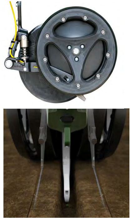
Figure 1. Conceal® placement 3" away from seed furrow and 1.5" deep
