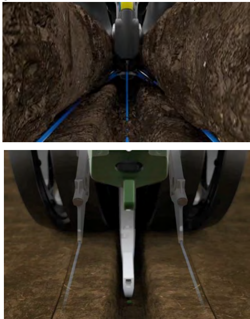
Figure 1. Conceal® and FurrowJet® Fertility Placement
