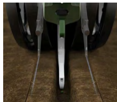
Figure 1. Conceal® placement 3" away from seed furrow and 1.5" deep
