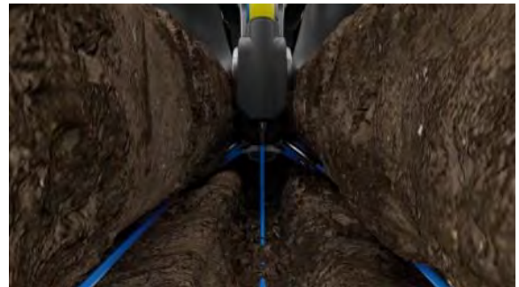
Figure 2: FurrowJet® Dual-Band Wings Fracturing Side-Walls
