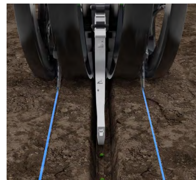
Figure 1. Conceal® placement 3" away from seed furrow and 1.5" deep
