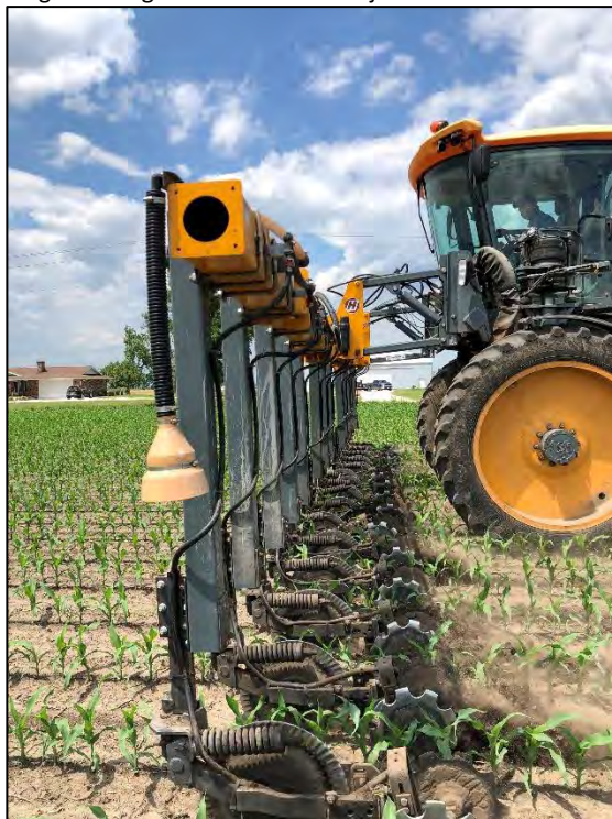
Figure 1. High Pressure Nozzle Injection with Sealers
