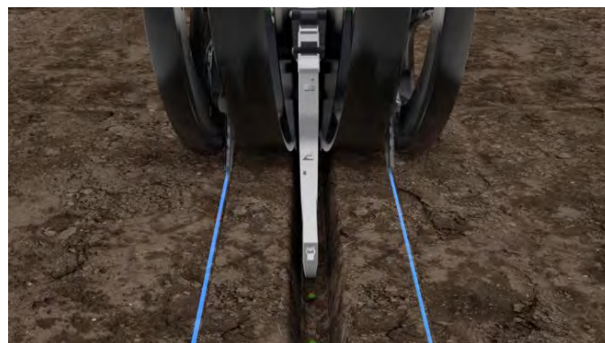
Figure 2. Conceal® Dual Placement 3" from Seed Trench
