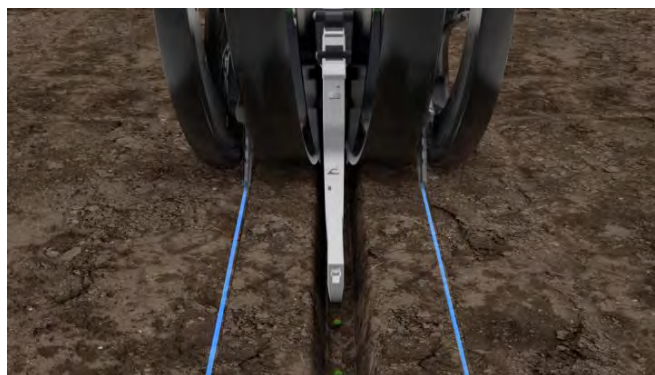
Figure 7. Conceal® Dual Placement 3" from Seed Trench
