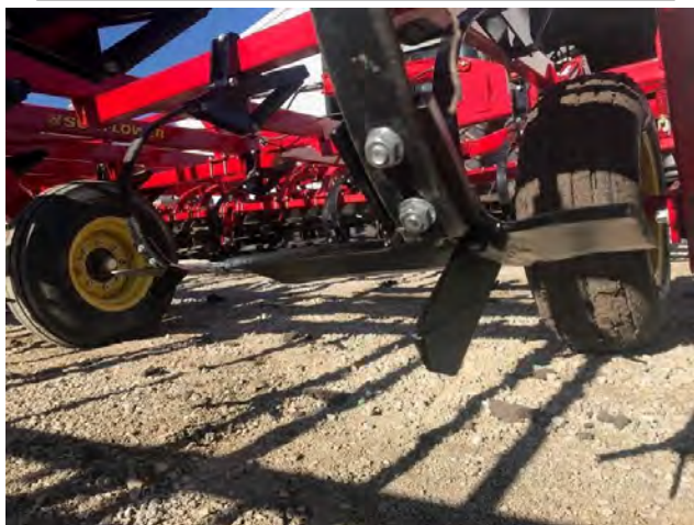
Figure 3. Finish™ Line Sweeps on 9" Spacing
