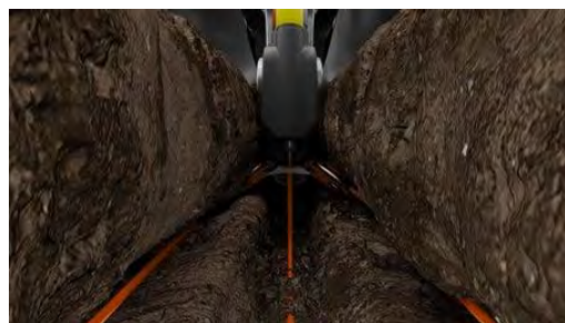
Figures 2-3: FurrowJet® Dual-Band Wings Fracturing Sidewalls
