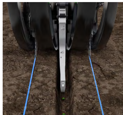
Figure 2. At-Plant Conceal Dual Band Nitrogen
