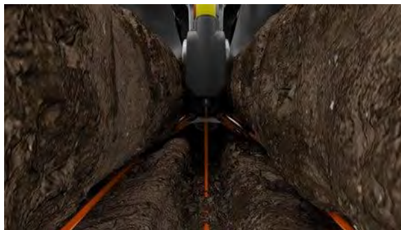
Figure 2: FurrowJet® Dual-Band Wings Fracturing Side-Walls
