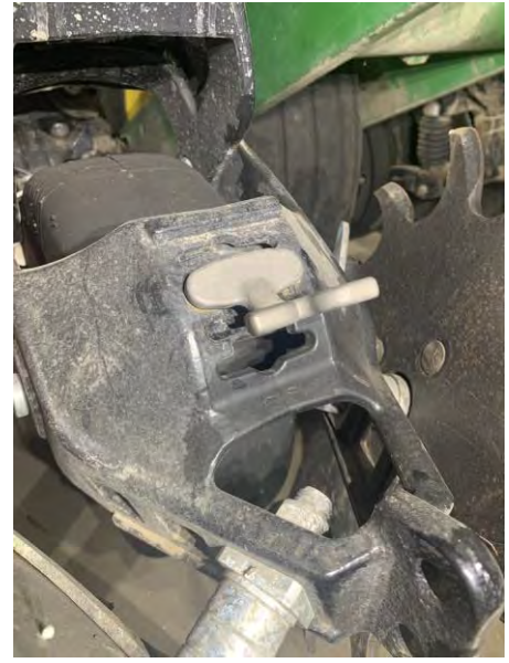
Figure 4. Reveal™ Depth Adjustment in Notch 1
