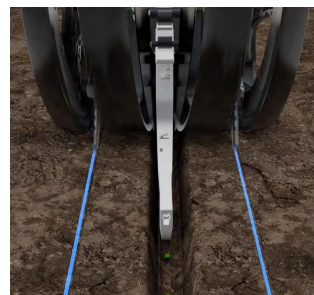
Figure 2. Conceal® Dual Placement 3" from Seed Furrow, 1.5" in Depth
