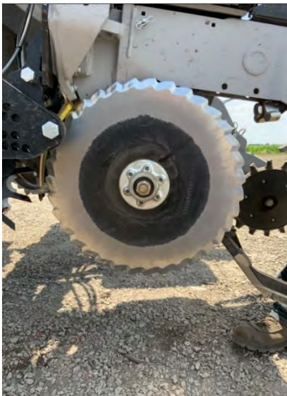
STP disc installed on Harvest International® planter
