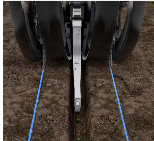
Figure 1. Conceal Single or Dual Placement 3" from Seed Trench, 1.5" in Depth
