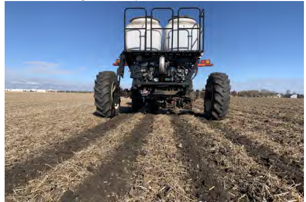
Figure 2. Strip-Till Banded Fertilizer
