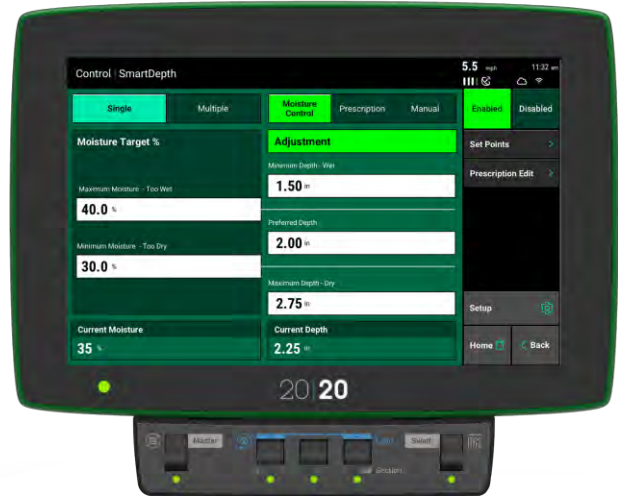
Figure 5. SmartDepth® Customization Screen
