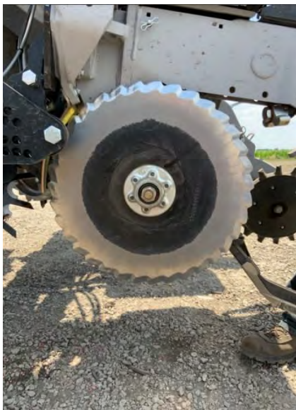
STP disc installed on Harvest International® planter
