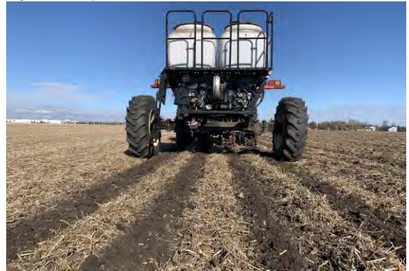
Figure 2. Strip-Till Banded Fertilizer
