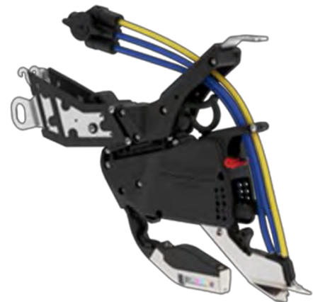
Figure 3. Conceal Dual Placement 3" from Seed Trench
