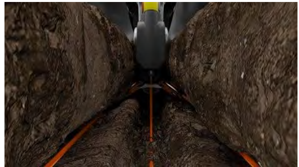
Figure 2: FurrowJet® Dual-Band Wings Fracturing Sidewalls
