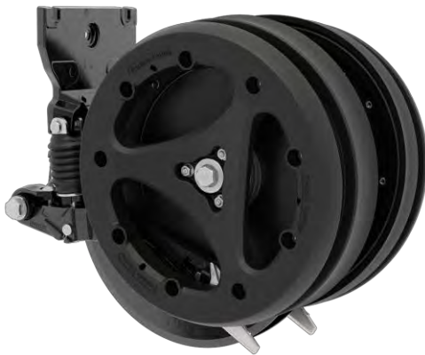
Figure 1. Conceal System Knife Design within Gauge Wheel
