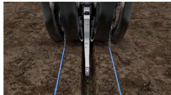
Figure 3. Conceal Dual Placement 3" from Seed Trench
