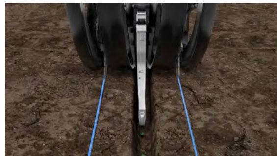
Figure 5. Conceal Dual Placement 3" from Seed Trench
