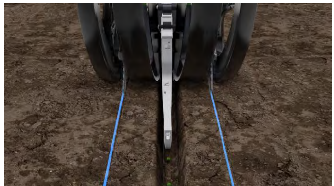
Figure 2. Conceal Dual Placement 3" from Seed Trench
