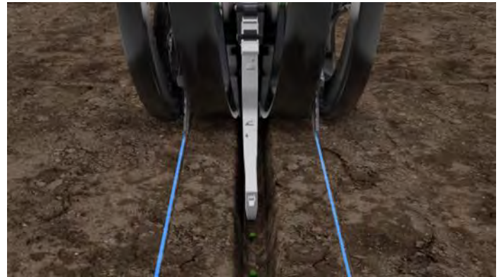
Figure 2. Conceal® Dual Band Placement
