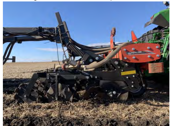
Figure 3. KUHN® Krause® strip-till unit
